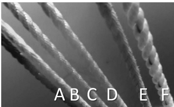
Fig. 11. Grayscale video still frame of black (A), blue (B), green (C), yellow (D), orange (E) and white (F) ropes at 5 m of water depth, an approximate mid-water column location. Differences in hue and contrast with the background are evident.
